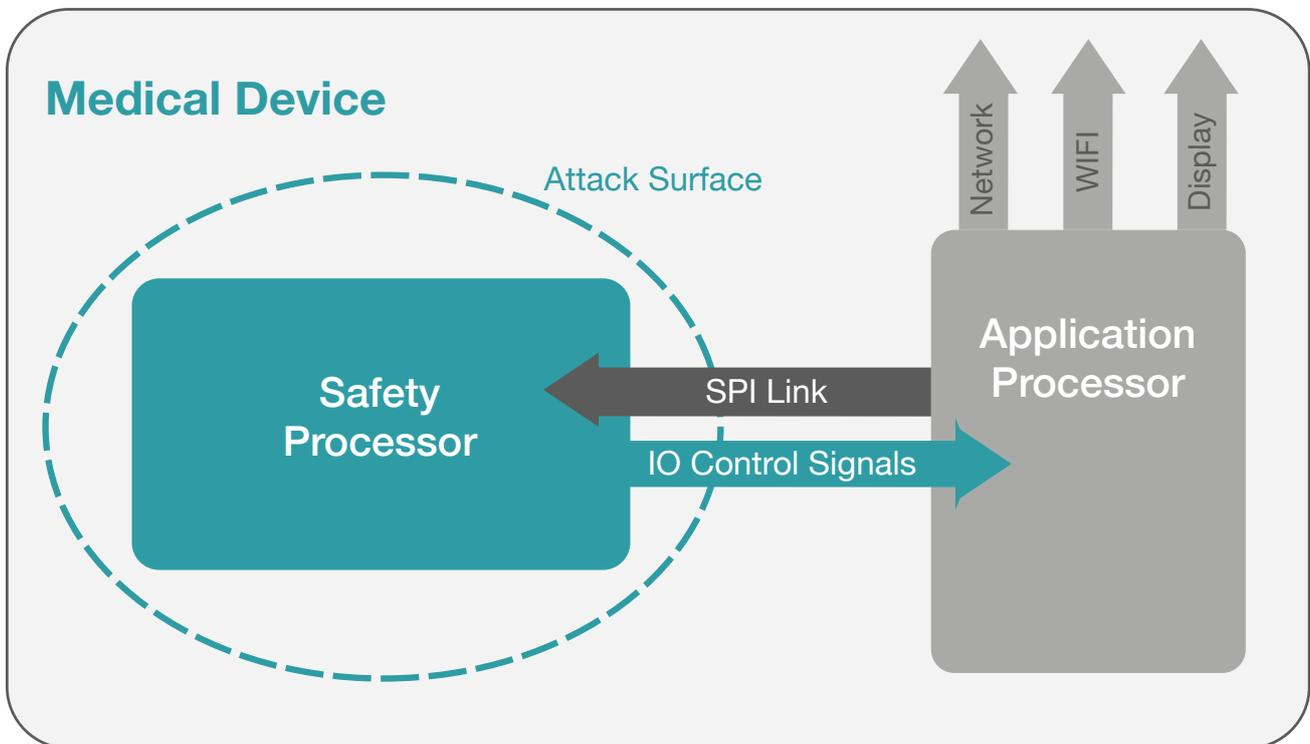
Figure 2. Potential attack surface for a dual core embedded medical device
